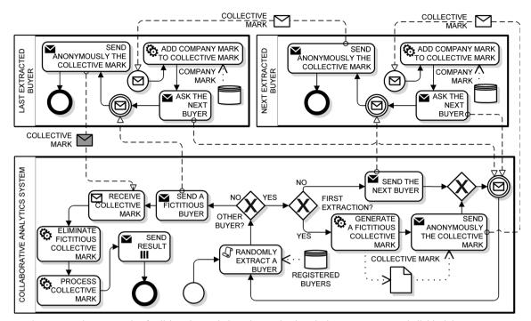
Fig. 9 DLIWORP approach: an example of collaborative analytics using marker-based stigmergy to preserve individual data source
