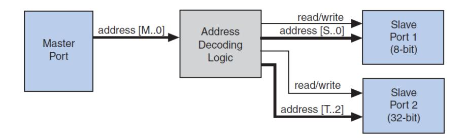
The address decoding logic is controlled by the Base address setting in the SoPC Builder
