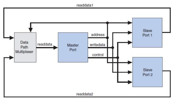
• In SOPC Builder, the generation of data path multiplexing logic is specified using the connections panel on the System Contents tab
