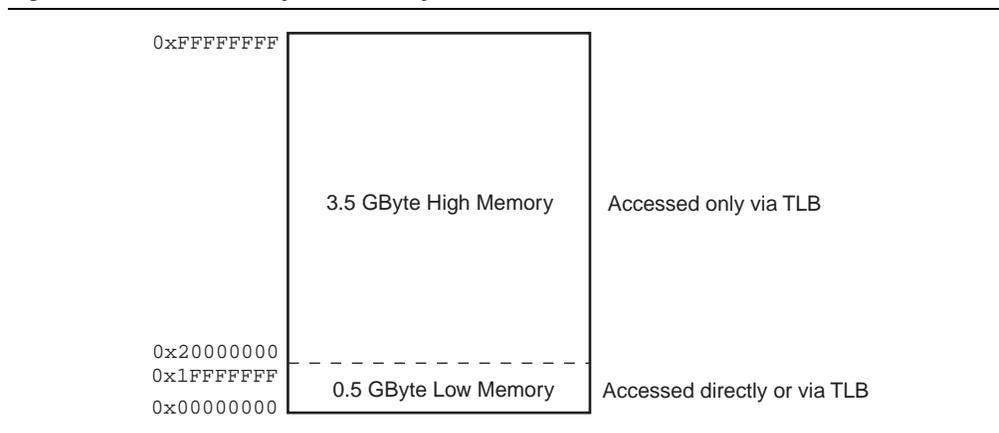
High physical memory can only be accessed through the TLB. Any physical address in low memory (29-bits or less) can be accessed through the TLB or by bypassing the TLB. When bypassing the TLB, a 29-bit physical address is computed by clearing the top three bits of the 32-bit virtual address.
