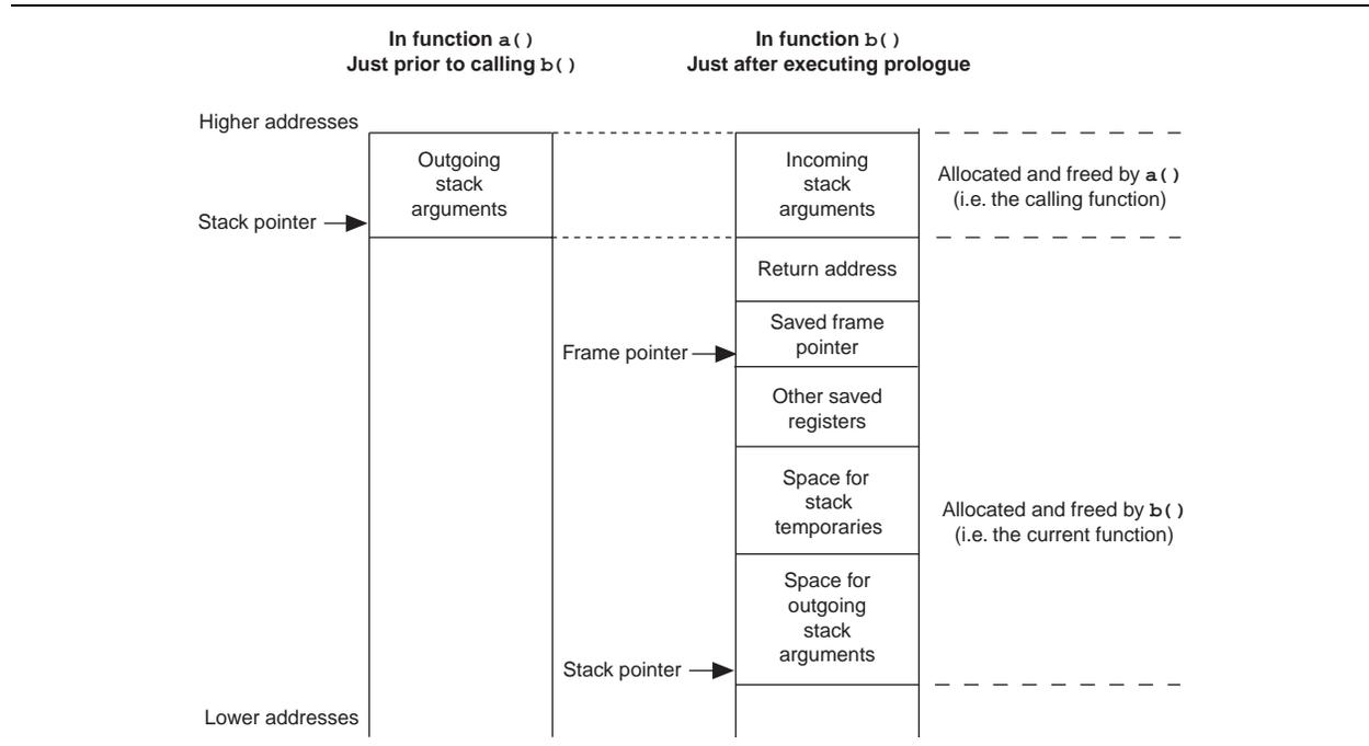
Each section of the current frame is aligned to a 32-bit boundary. The ABI requires the stack pointer be 32-bit aligned at all times.
