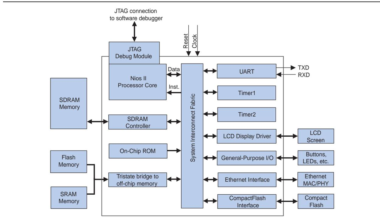
If the prototype system adequately meets design requirements using an Altera-provided reference design, you can copy the reference design and use it without modification in the final hardware platform. Otherwise, you can customize the Nios II processor system until it meets cost or performance requirements.
