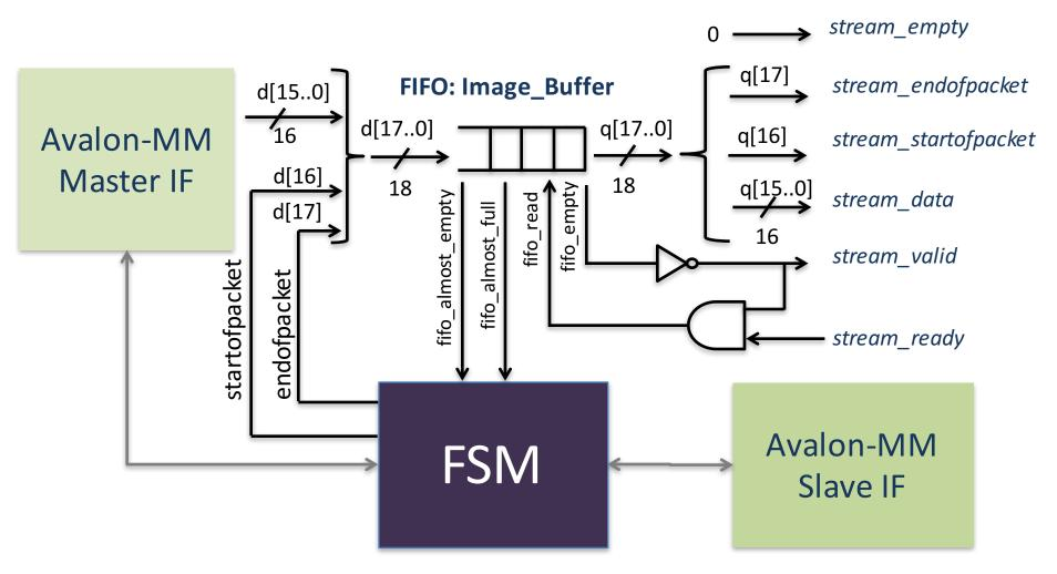
FSM manages Avalon-MM Master transfers to keep FIFO level between almost-full and almost-empty VGA F
