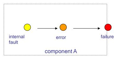
A fault causes an error in the internal state of the system. The error causes the system to fail
