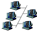
shared wire (e.g., cabled Ethernet)
