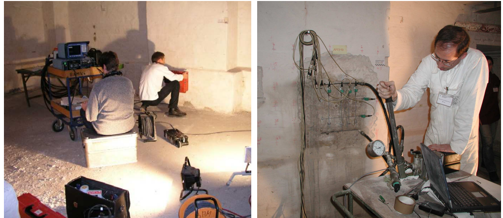
Figure 2. Altes Museum Berlin, Radar (left) and flat jack tests.
