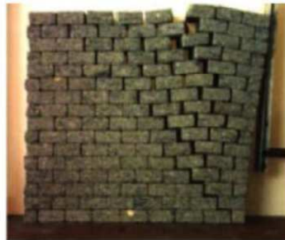
Figure 5.21 Masonry walls under uniform vertical and horizontal accelerations: (a) view of the walls, (b) system of application of the load adopted by Ceradini (1992).
