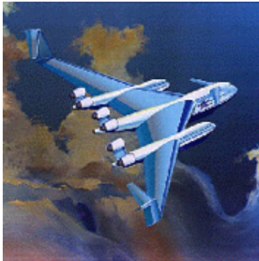
Figure: C-Wing: an example of non-planar wing system.
