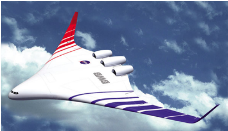
Figure: BWB tries to minimize wetted area.
