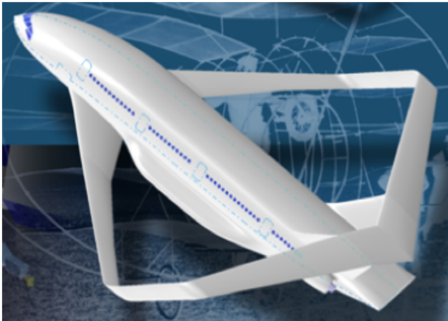
Figure: Based on the Best Wing System by Prandtl: the induced drag is minimum.
