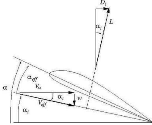
**Fig. 1:**  $\alpha$ -geometric angle of incidence,  $\alpha_i$ -angle of induced velocity,  $\alpha_{eff}$ -actual angle of incidence.
