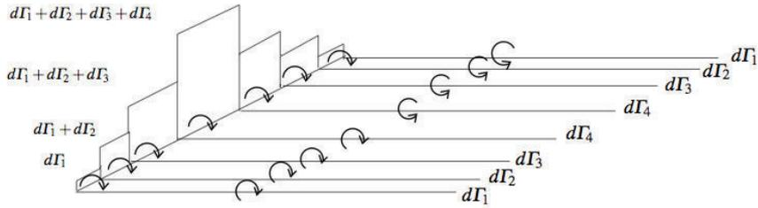
**Fig. 2:** Vortices on the wing wake: on the lifting line, the difference between vortices (or circulation) equals the free vortices detaching from trailing edge.
