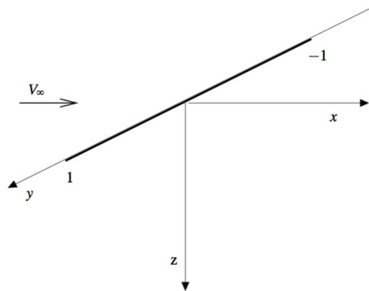
**Fig. 3:** Reference frame of the lifting line wing.
