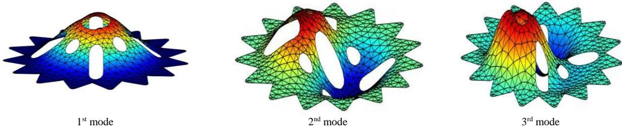
Figure 4. First three mode shapes of the gear-shaped plate with lay-up  $[0^\circ/45^\circ]$  and clamped edges ( $h/a=0.1$ )
