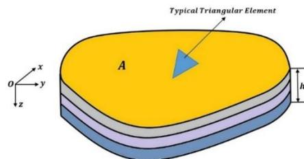
**Figure 1.** Laminated composite plate with arbitrary lay-up and in-plane shape
