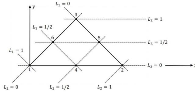
**Figure 2.** Area coordinates for obtaining the shape functions [11]
