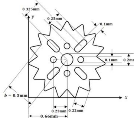
Figure 3. Gear-shaped plate
