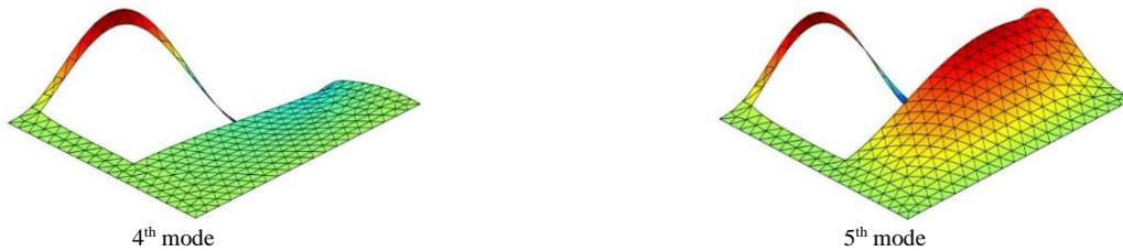
**Figure 6.** First five mode shapes of a composite car door-shaped plate with lay-up  $[45^\circ/60^\circ/60^\circ/45^\circ]$  and CCF boundary conditions ( $h/a=0.1$ )
