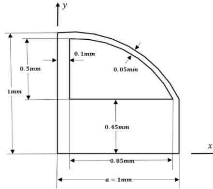
**Figure 5.** Laminated composite plate in the shape of a car door
