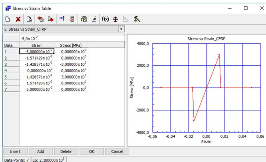
Figure 19: Stress-strain curve for CFRP laminates
