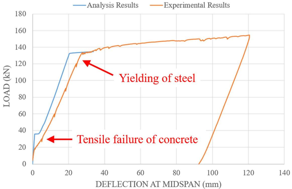
Figure 20: Comparison between the theoretical and experimental load-deflection curves – Specimen 1
