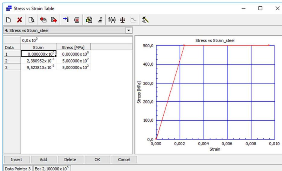
Figure 18: Stress-strain curve for steel
