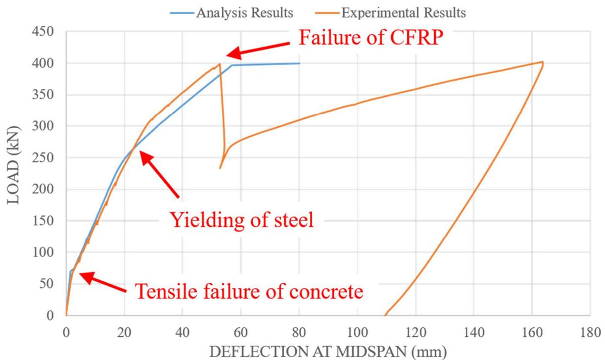
Figure 21: Comparison between the theoretical and experimental load-deflection curves – Specimen 3
