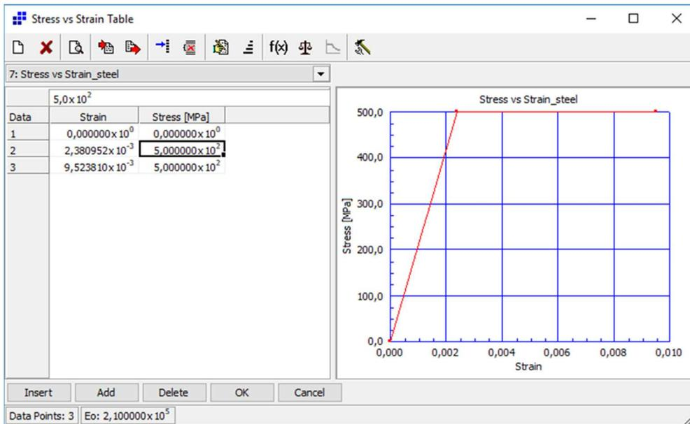
Figure 7: Stress-strain curve for steel
