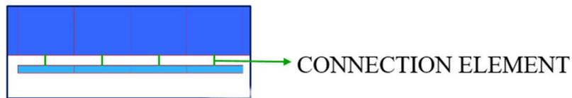
Figure 11: Connection between CFRP laminates and concrete
