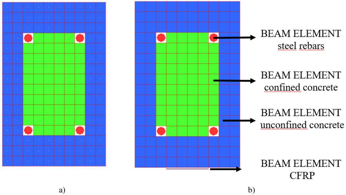
Figure 10: FE models for a) beam 1; b) beam 2
