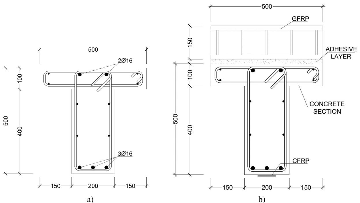
Figure 1: Prototype reinforced concrete beam: a) un-strengthened; b) strengthened
