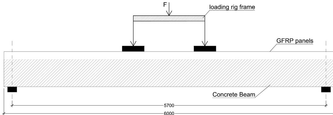
Figure 2: Four-point bending test configuration
