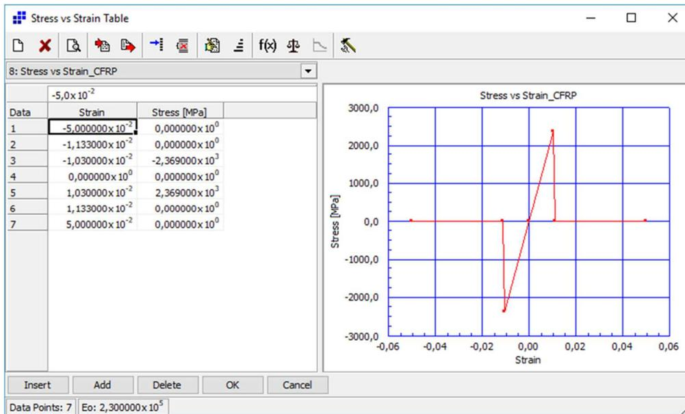
Figure 8: Stress-strain curve for CFRP laminates
