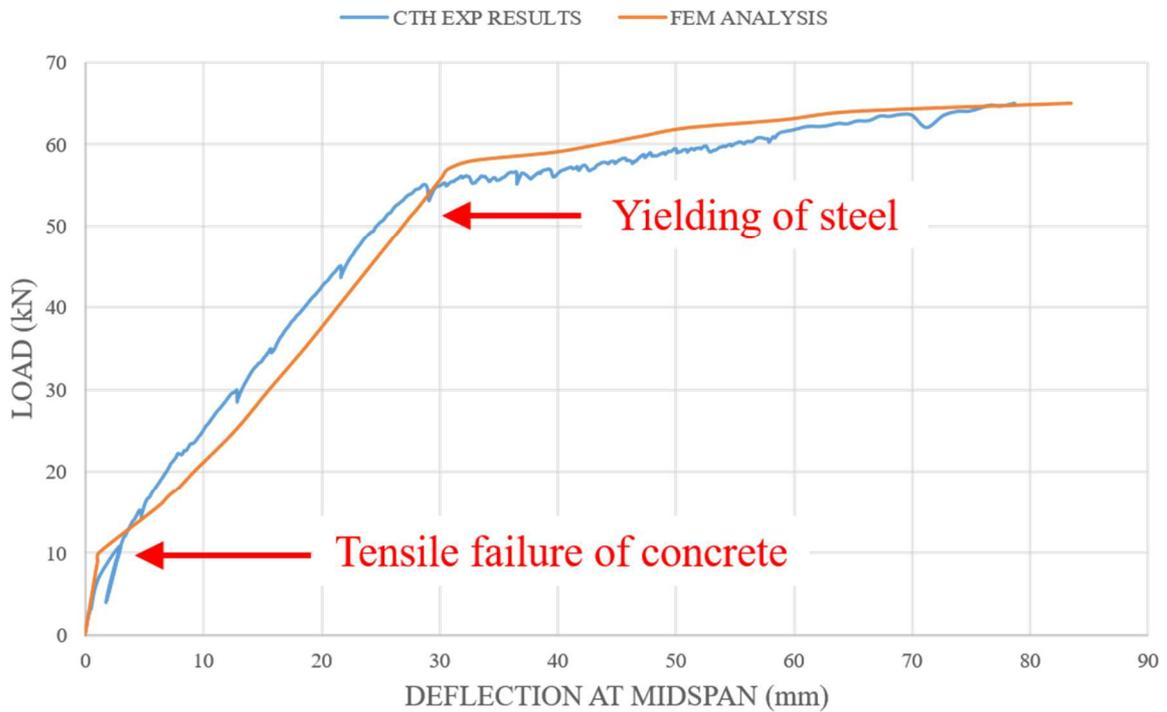
Figure 12: Comparison between the theoretical and the experimental load-deflection curves – Beam 1
