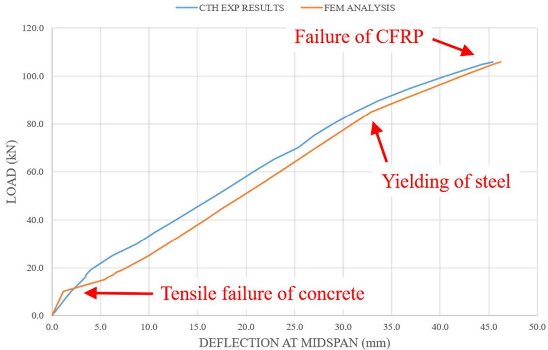
Figure 13: Comparison between the theoretical and the experimental load-deflection curves – Beam 2
