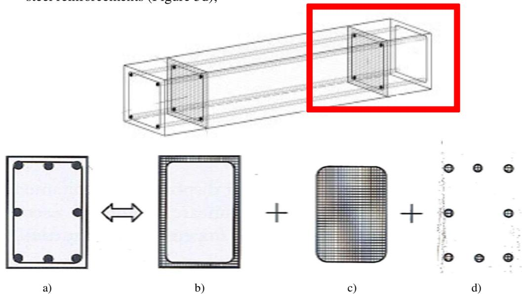
Figure 5: a) Concrete section; b) Unconfined concrete; c) Confined concrete; d) Steel reinforcements
