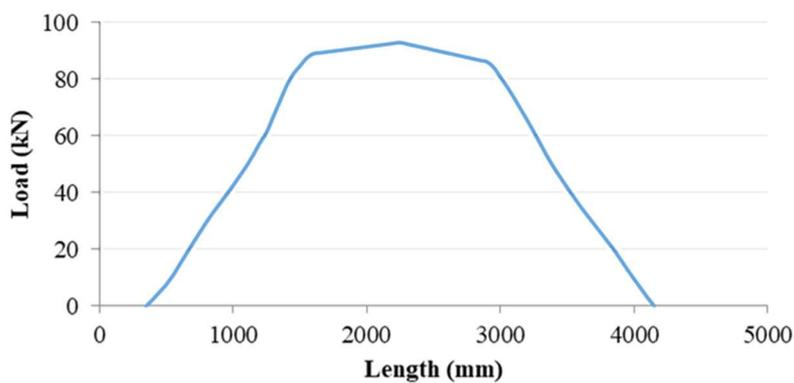
Figure 9: Pre-stress distribution for CFRP laminates
