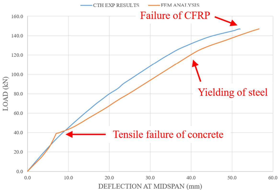
Figure 14: Comparison between the theoretical and the experimental load-deflection curves – Beam 3
