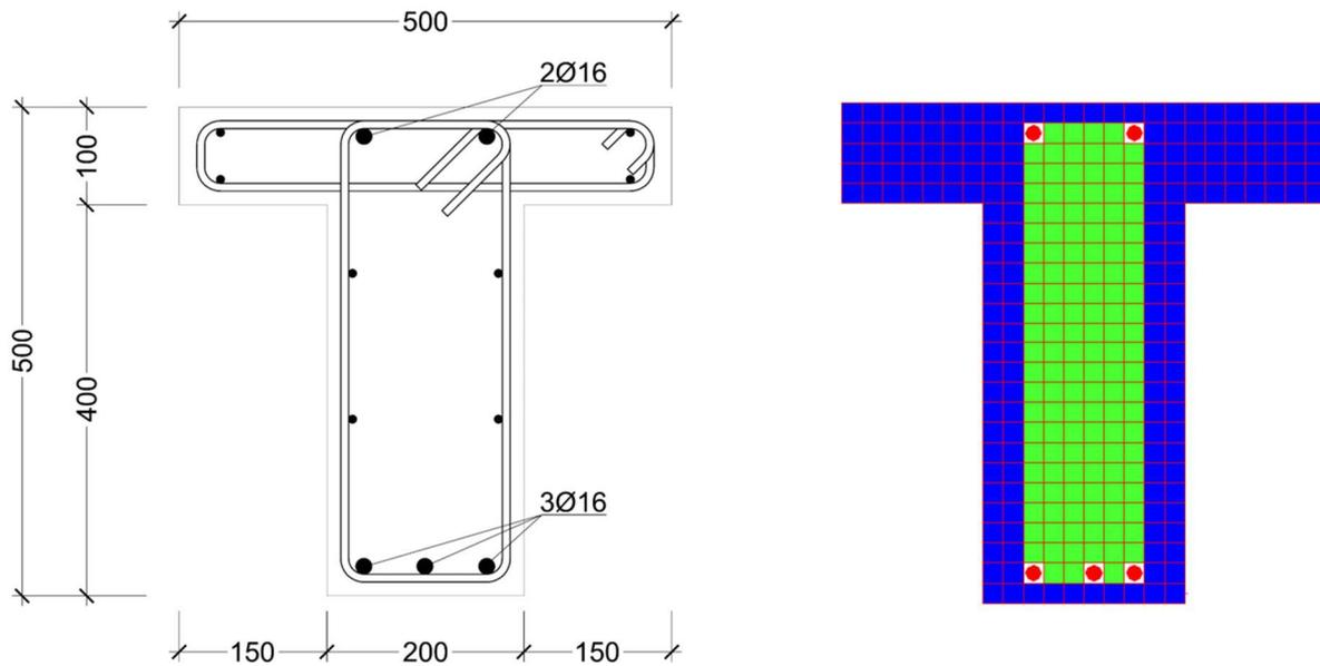
Figure 15: FE cross section of specimen 1
