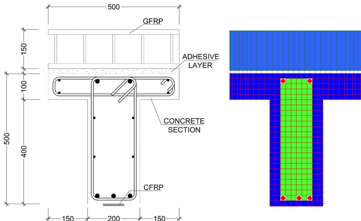
Figure 16: FE cross section of specimen 2
