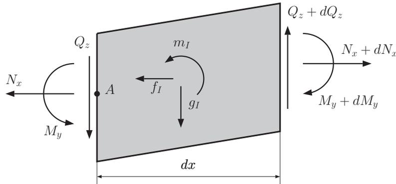
Figure 6: Equilibrium of a differential element of the beam.
