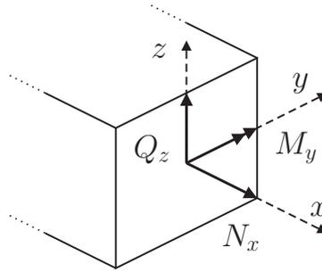
Figure 4: Positive resultant forces and bending moment.
