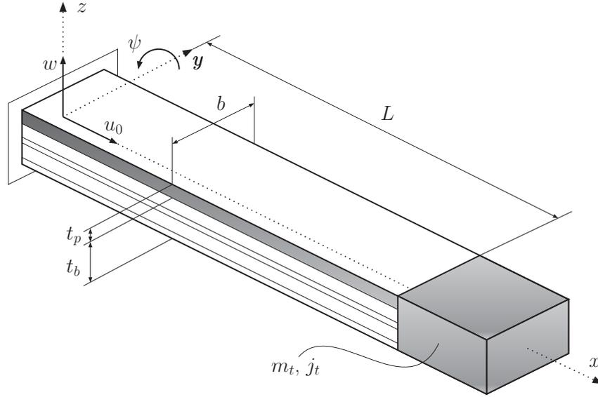
Figure 3: Piezoelectric cantilever beam.
