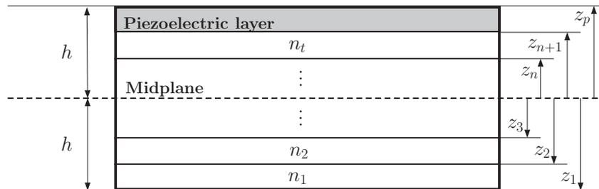
Figure 5: Geometry of laminated composite beam section.
