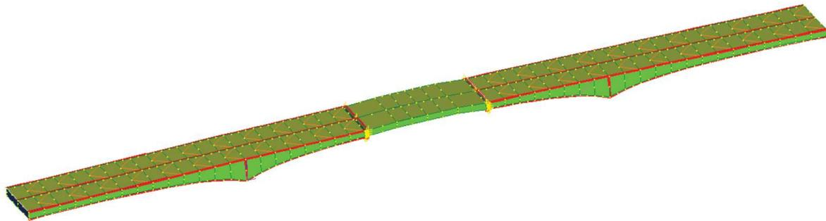
Figure 2: Finite element model of the Cittadella bridge.
