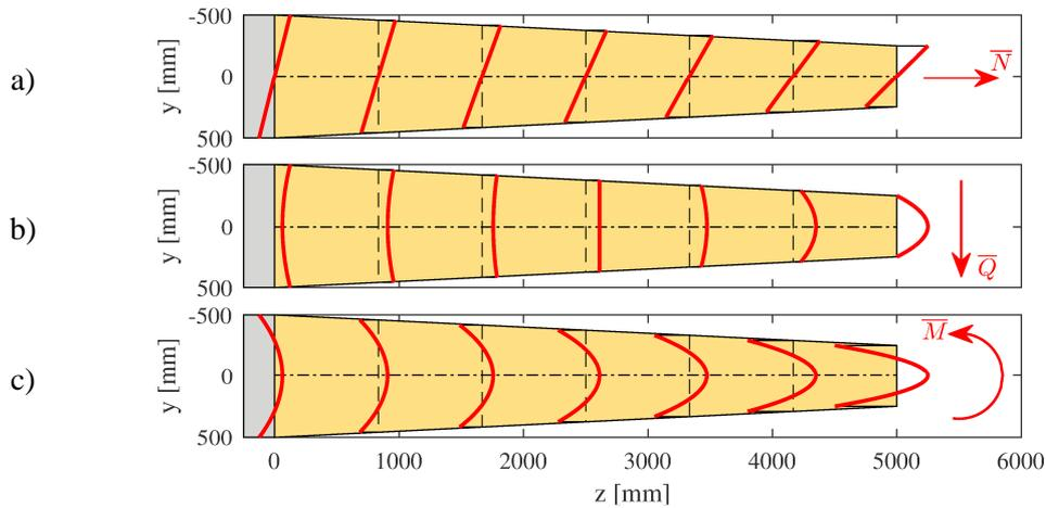
Figure 2: shear stresses under: a) axial force; b) shear force; c) bending moment.
