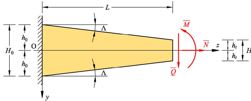
Figure 1: tapered cantilever beam subjected to tip loads.
