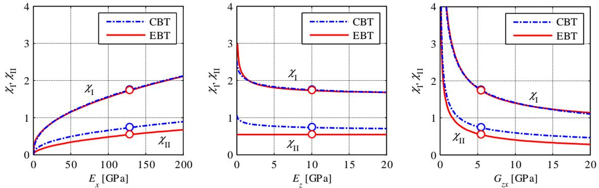
Figure 1: Crack length correction parameters as functions of the elastic moduli of a homogenous orthotropic specimen (from [9]).
