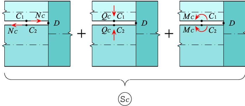
Fig. 5: Crack-tip forces in system  $S_C$ .
