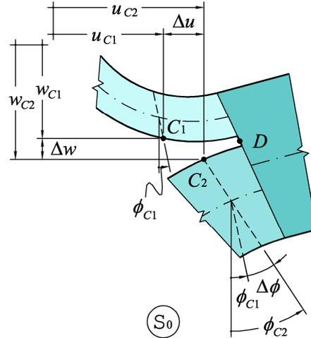
**Fig. 4:** Crack-tip relative displacements in system  $S_0$
