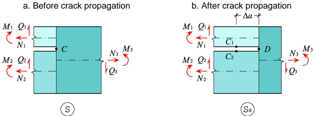
Fig. 3: Elementary segment of the laminate in the neighbourhood of the crack tip
