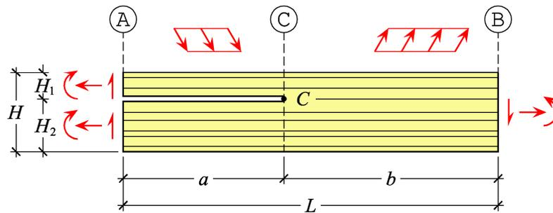
Fig. 1: The delaminated laminate subjected to concentrated and distributed loads
