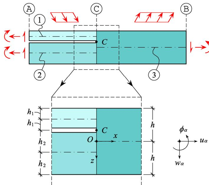
Fig. 2: The delaminated laminate as an assemblage of three laminated beams
