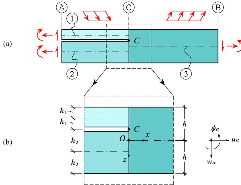
Figure 2: (a) The delaminated laminate as an assemblage of three laminated beams;
