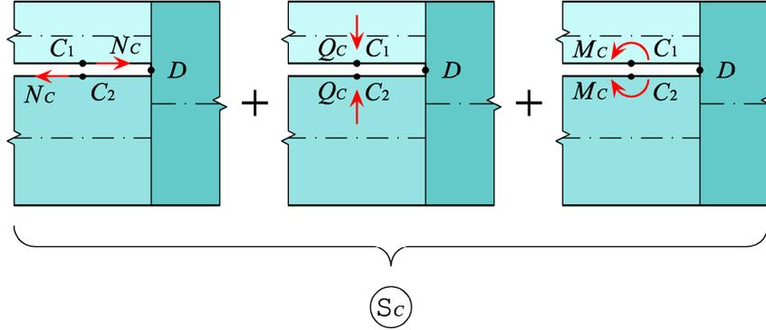
Figure 5: Crack-tip forces in system  $S_C$ .
