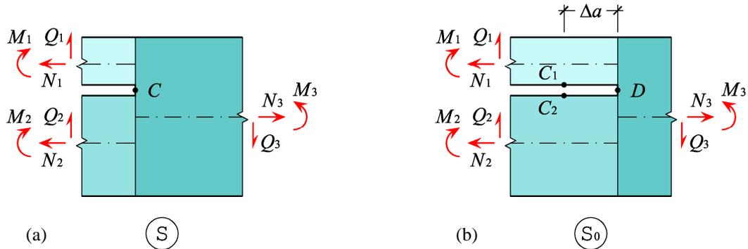
Figure 3: Elementary segments of the laminate in the neighbourhood of the crack tip:
