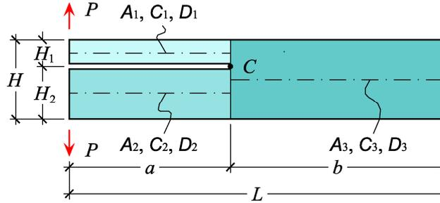
Figure 6: The asymmetric double cantilever beam (ADCB) test.
