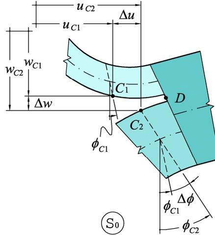
Figure 4: Crack-tip relative displacements in system  $S_0$ .
