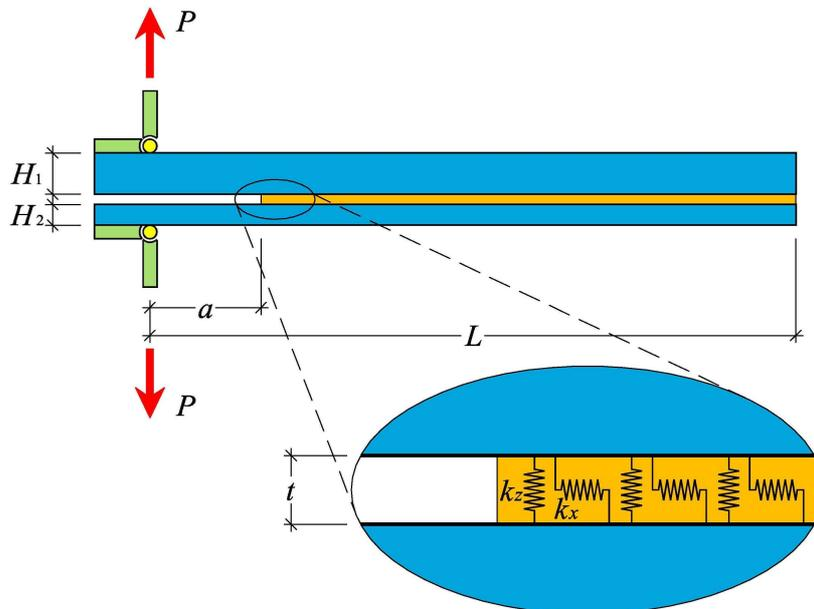
Fig. 1 : The mechanical model of the ADCB test.
