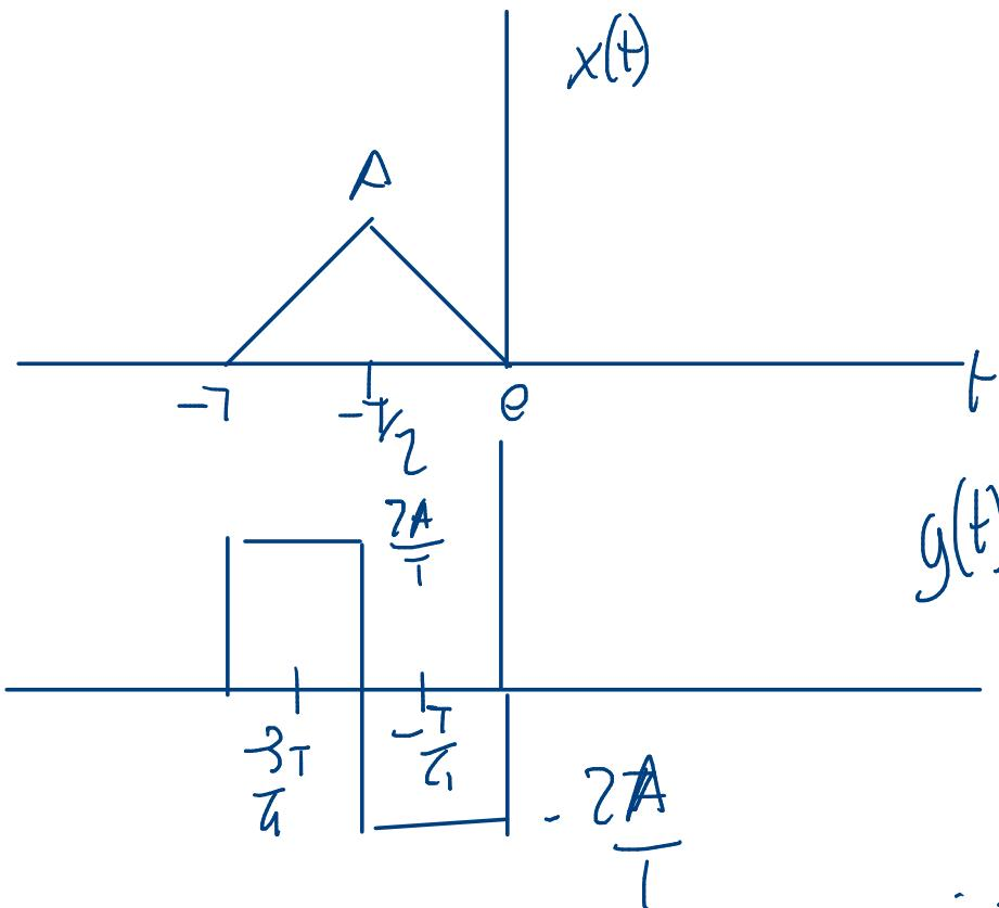
$$g(t) = \frac{2A}{T} \text{Vect} \left( \frac{t+3T}{\frac{T}{4}} \right) - \frac{2A}{T} \text{Vect} \left( \frac{t+\frac{T}{4}}{\frac{T}{2}} \right)$$
