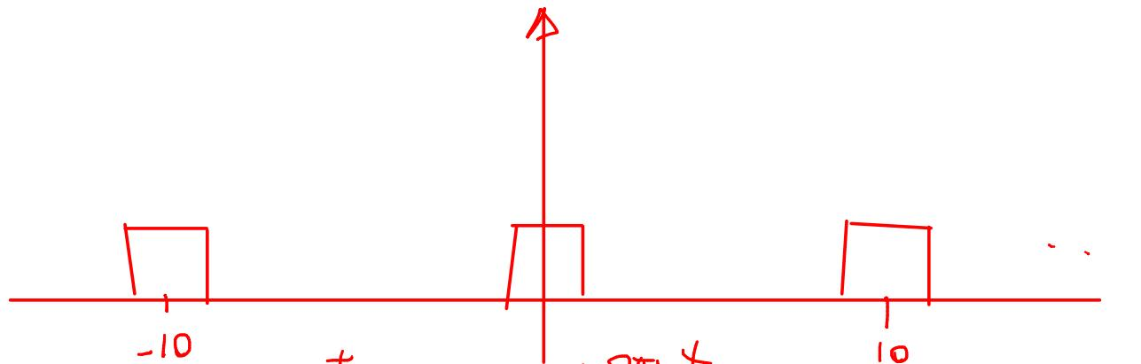
$$S_n = \frac{1}{T_0} \int_{-\frac{T_0}{2}}^{\frac{T_0}{2}} s(t) e^{-j2\pi n \frac{t}{T_0}} dt$$
