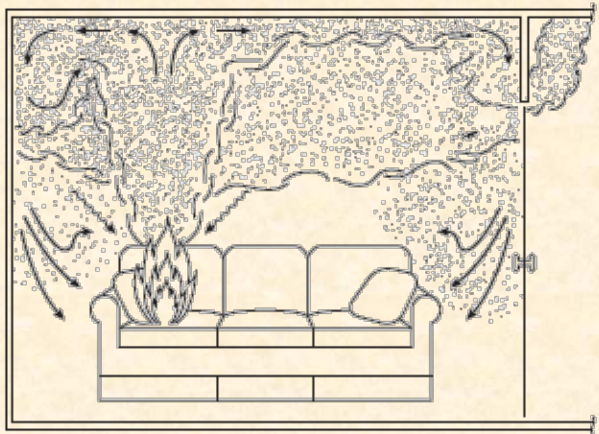
Figure 3-10.6. Further "smoke filling."
