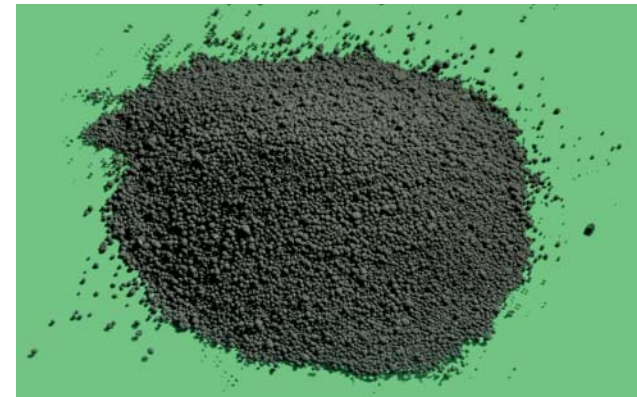
Carbon black is a fine powder obtained by the incomplete combustion of petroleum oils.
