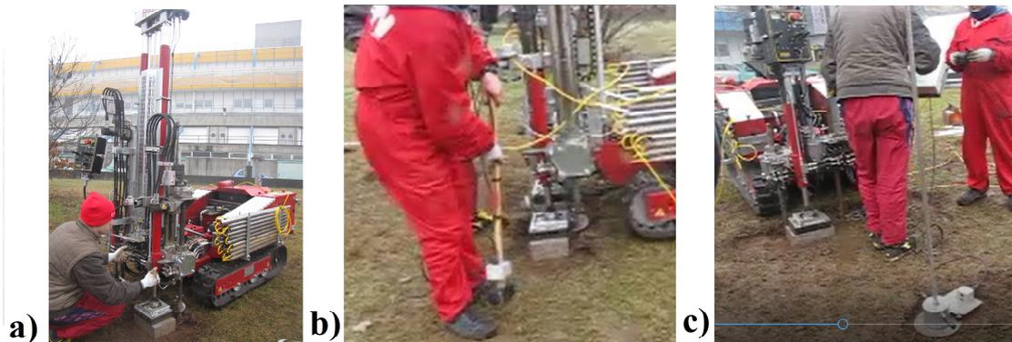
Figure 7 SCPT set-up at the University of Pavia campus. A) Pagani TG63 – 200 penetrometer; B) manual hammer of 5 kg hitting the aluminium blocks; C) sledgehammer.
