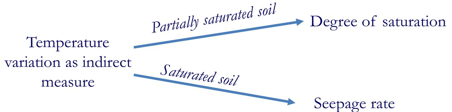
**heat-pulse method:** coupling electric cable to the fiber, the electric cable heats the fiber, measuring the heating time and the difference between zones it is possible to assess the flux of water around the cable (areas with higher water transport will rise to lesser temperatures)
