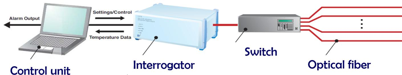
The interrogator sends a laser beam inside the fiber; then it reads the backscatter signal reconstructing the longitudinal profile of temperature.
