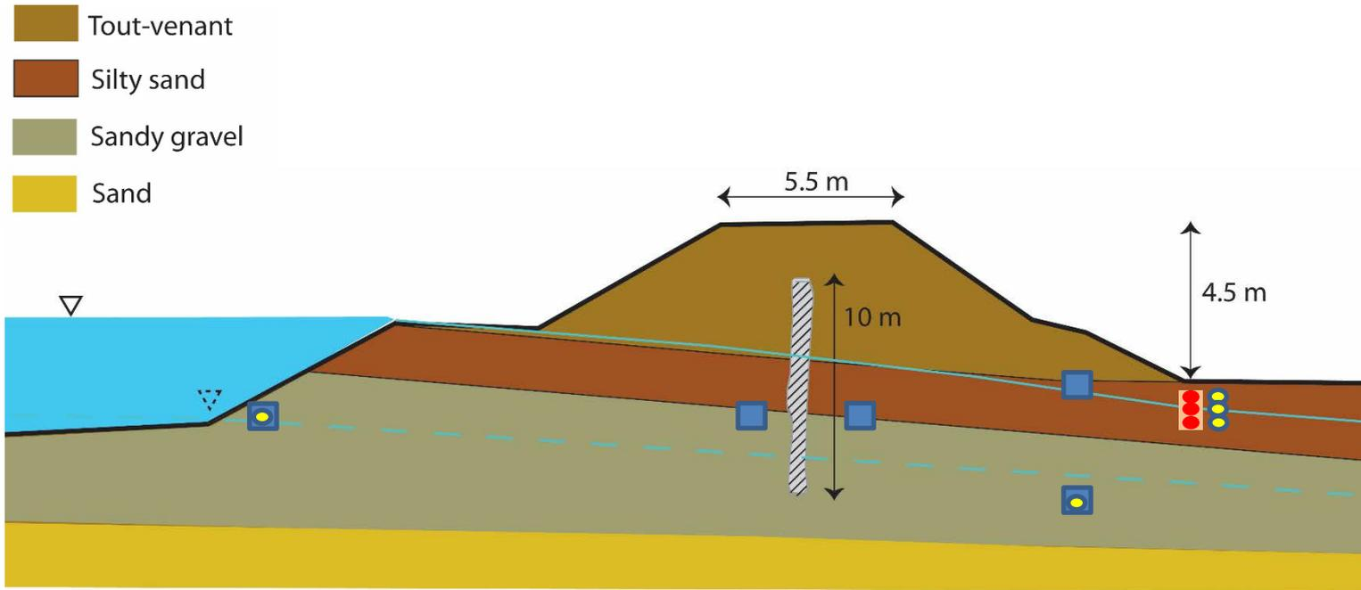
Three levels of optical fiber about 50 cm apart along the vertical
