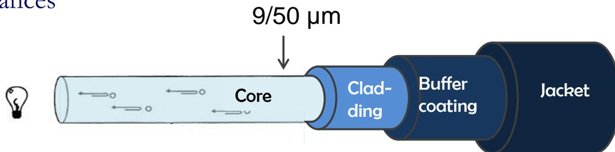
When a light impulse is injected in an optical fibre a backscattered light is generated by each point along the fibre. The spectrum of the backscattered light carries information about the local status of the fiber
