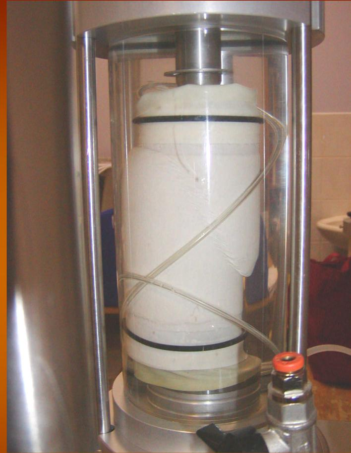
**Fig 14. Dense sand sample, which  $H/D = 2$ , in improved triaxial test apparatus**
