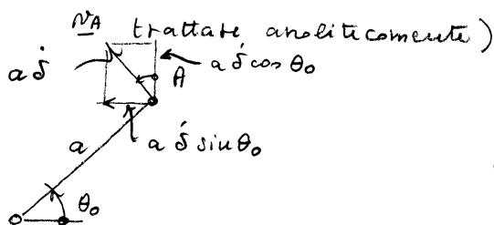
$$\underline{v}_A = \underline{v}_B = \underline{v}_C = \underline{v}_G = -r \sin \theta_0 \dot{\delta} \underline{i} + r \cos \theta_0 \dot{\delta} \underline{j}$$
