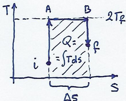
PERCHÈ SIA MASSIMO  $\int T ds$  BASTA SEMPLICEMENTE CHE SIA SCAMBIATO (ASSORBITO DAL GAS) CALORE ALLA TEMPERATURA PIU' ALTA POSSIBILE.
