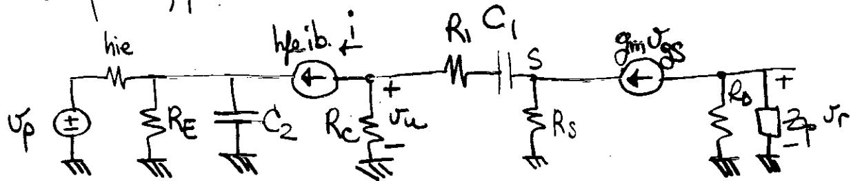
$$\left| \frac{i}{i_p} \right|_0 = \frac{h_{fe}}{h_{ie} + (h_{fe} + 1)R_E} = \frac{300}{605840} = 0.495 \cdot 10^{-3} \Omega^{-1} = \xi_0$$
