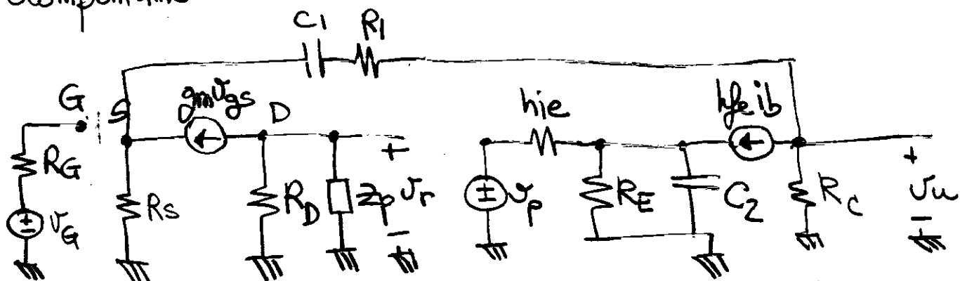
$$Z_p = \frac{h_{ie} + R_E(h_{fe}+1)}{R_E C_2 s + 1} = \frac{h_{ie} + R_E h_{fe} + R_E C_2 s h_{ie}}{1 + R_E C_2 s} =$$
