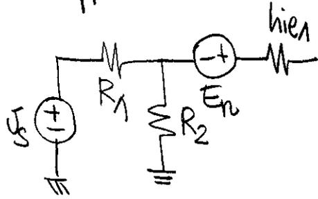
$$A_{f_{E_n}} = A_f \frac{R_1 + R_2}{R_2}$$
