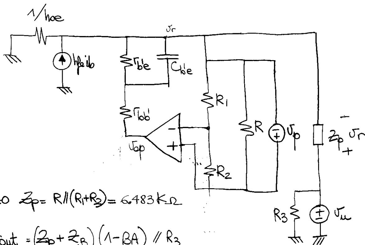
$$\rho = 0 \quad Z_p = R_1 \parallel (R_1 + R_2) = 6.483 \text{ k}\Omega$$
