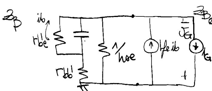
$$z_{B0} = \frac{(r_{be} + r_{bb})}{h_{fe} + 1} \parallel \frac{1}{h_{oe}} \approx \frac{r_{be} + r_{bb}}{h_{fe} + 1} = 26.2 \Omega$$
