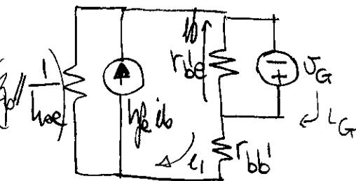
$$i_1 = \frac{v_G \left[ 1 + \frac{h_{fe}}{r_{be}} \left( z_p \parallel \frac{1}{h_{oe}} \right) \right]}{r_{bb} + \left( z_p \parallel \frac{1}{h_{oe}} \right)}$$
