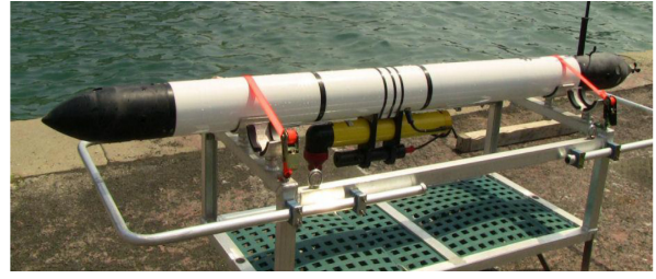
Figure 2. Fòlaga AUV with the UAN module with the acoustic modem and CTD mounted at mid-vehicle.
