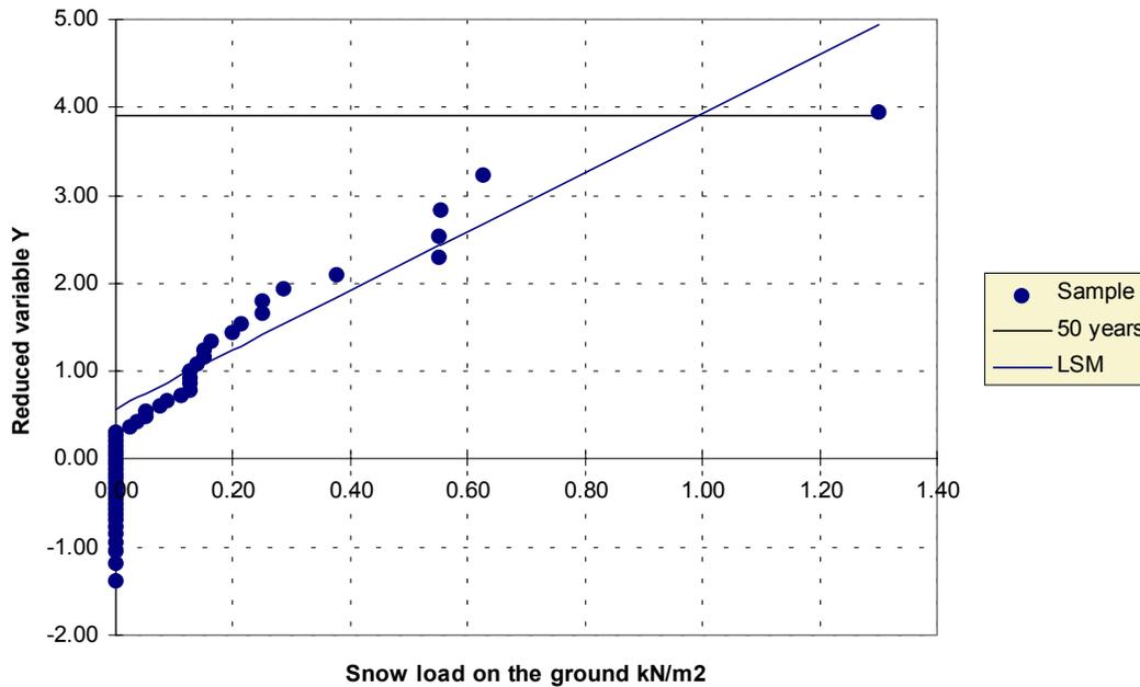
Figure 4.3 Extreme value plot in which a high value appears (Pistoia, 58 m a.s.l. - Italy)
