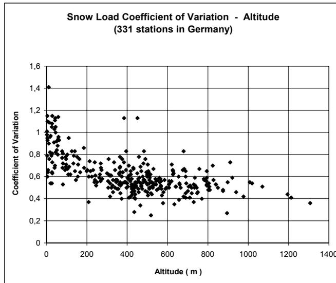
Figure 4.4: Coefficient of variation of snow loads for climatic stations in Germany
