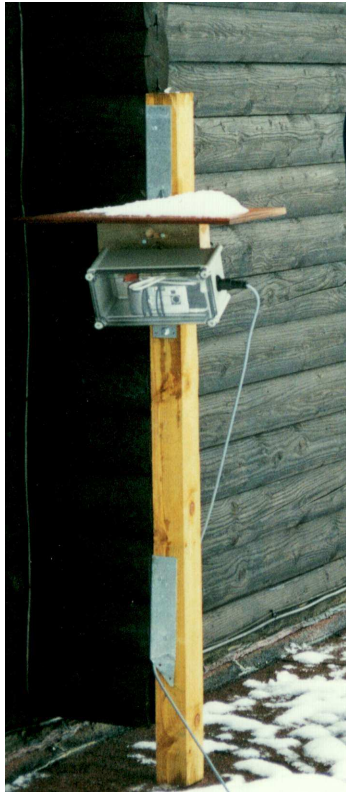
Figure A.8.2-3: Digital camera housed in a heated container
