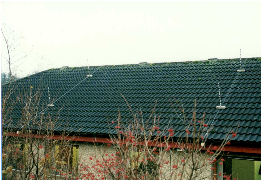
Figure A.8.2-2: BRE pressure pad system
