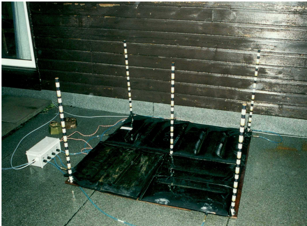
Figure A.8.2-2: BRE pressure pad system
