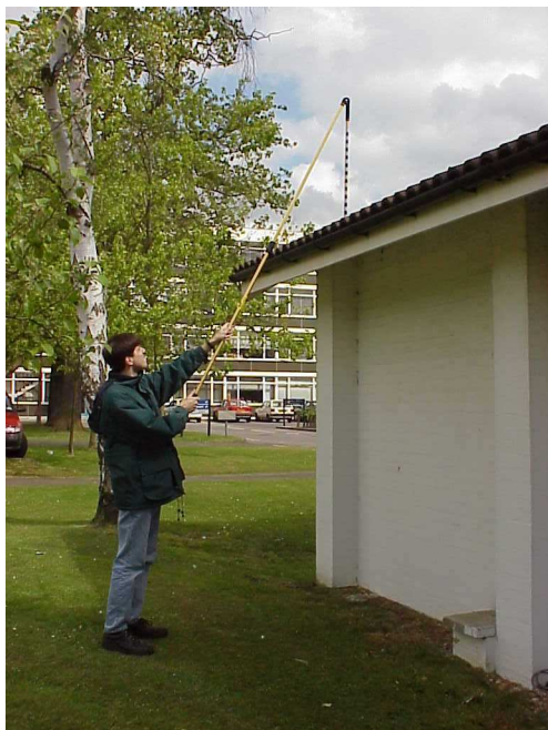
Figure A.8.2-4: BRE hand-held snow depth measuring system
