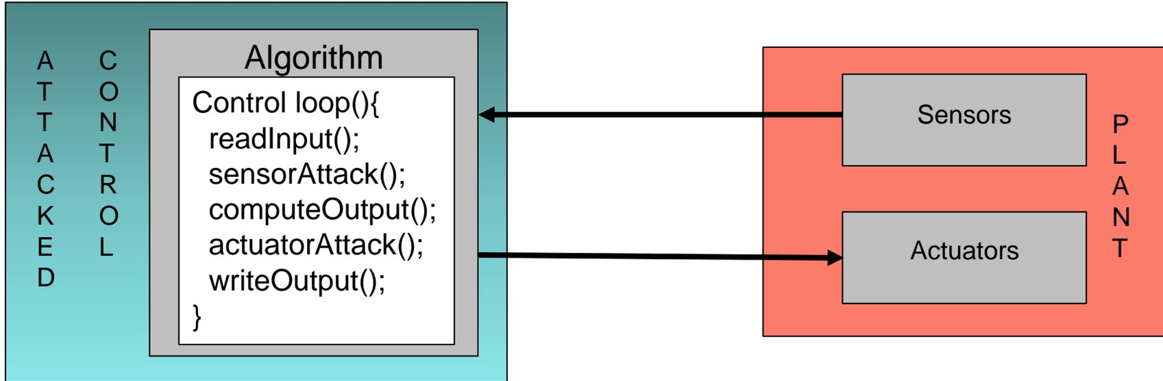
The behavior of the attack is implemented inside the control FMU
