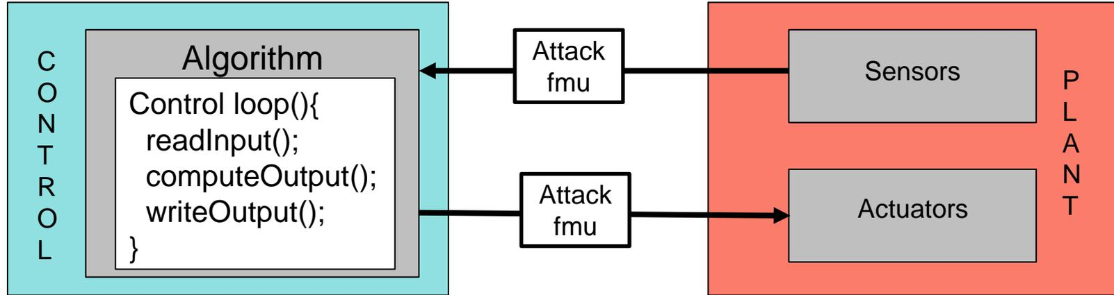
The behavior of the attack is implemented inside an external FMU added to the system
