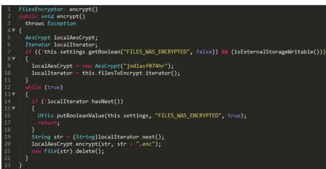
The class AesCrypt carries out the actual encryption and decryption of files.
