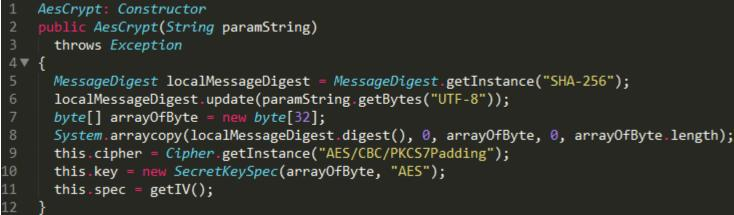
• This code snipped shows that the ransomware uses AES encryption using AES/CBC/PKCS7Padding.
