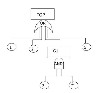
$\begin{array}{ll} \mbox{Minimal Cut Sets} \\ \mbox{Top} = \{1\}, \{2\}, \{3, 4\}, \{5\} \\ \mbox{S}_1 = \{1\} & \mbox{S}_2 = \{2\} & \mbox{S}_3 = \{3, 4\} & \mbox{S}_4 = \{5\} \end{array}$
