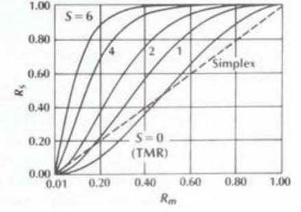
System with standby failure rate equal to 10% of on line failure rate
