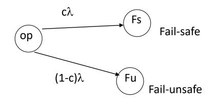
Modeling coverage in a Markov chain means that every un-failed state has two transitions to two different states, one of which is fail-safe, the other is fail-unsafe.
