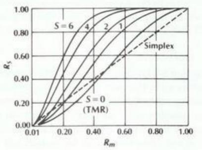
System with standby failure rate equal to on-line failure rate
