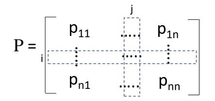
Each state of the Markov chain is a node Each p<sub>ij</sub> >=0 corresponds to a directed Edge from node i to node j
