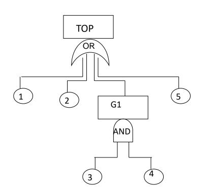
Q<sub>s</sub>(t) = probability that all components in the minimal cut set S are faulty
