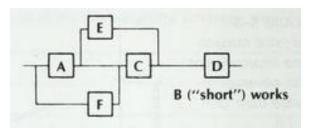
P(system works | B works) must be further reduced
