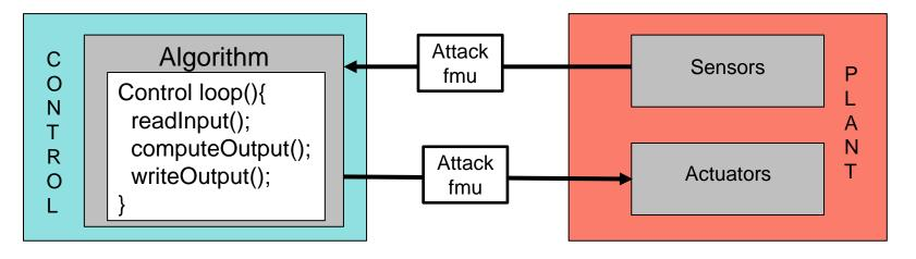
The behavior of the attack is implemented inside an external FMU added to the system
