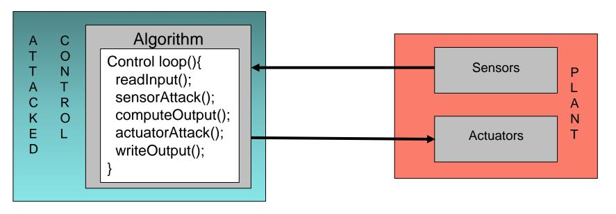
The behavior of the attack is implemented inside the control FMU
