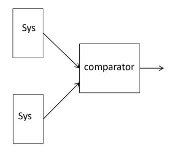
Assumption on faults is very important. most of the time single fault assumption
