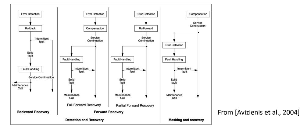
Solid faults: permanent faults whose activation is reproducible Elusive faults: permanent faults whose activation is not systematically reproducible (e.g, conditions that occur in relation to the system load, pattern sensitive faults in semiconductor memories, ...) Intermittent faults: transient physical faults + elusive development faults
