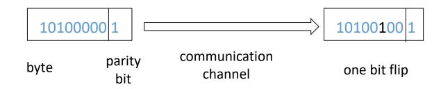
for each unit of data, e.g. 8 bits, add a parity bit so that the total number of 1's in the resulting 9 bits is odd
