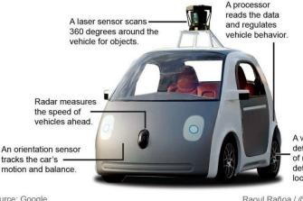
A wheel-hub sensor detects the number of rotations to help determine the car's location.
