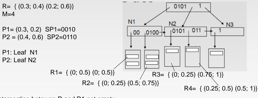
Intersection between R and R1 not empty Intersection between R and R4 not empty
