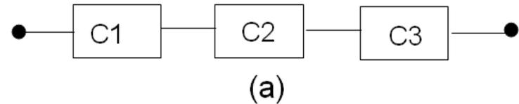
If each individual component  $i$  satisfies the exponential failure law with constant failure rate  $\lambda_i$ :
