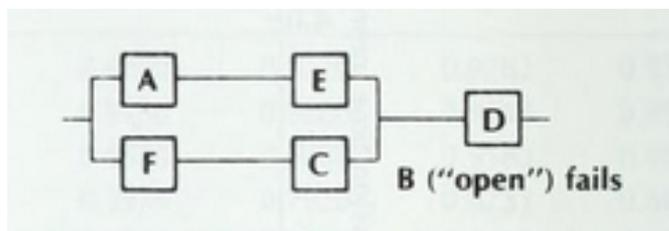
$$P(\text{system works} \mid B \text{ fails}) = \{ R_D [1 - (1 - R_A R_E) (1 - R_F R_C)] \}$$
