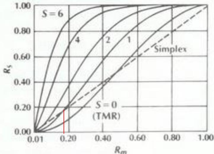
Figure 2. system with standby failure rate equal to 10% of on line failure rate
