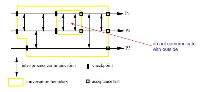
Example where three processes communicate within a conversation and the processes P1 and P2 communicate within a nested conversation
