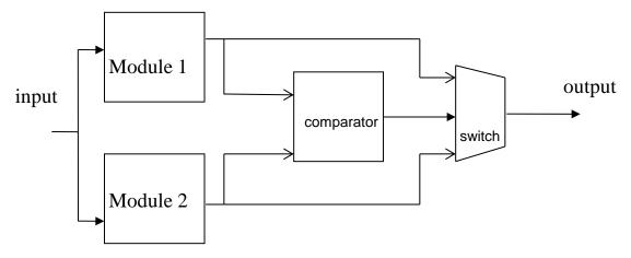
Sometimes named dual-modular redundancy
