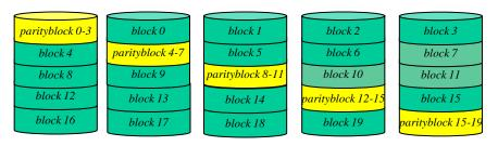
Level 6 instead of using parity, uses ECC
