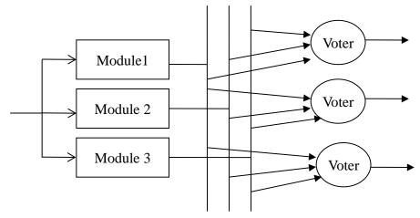
If triplicated output is desired, the single point of failure is removed
