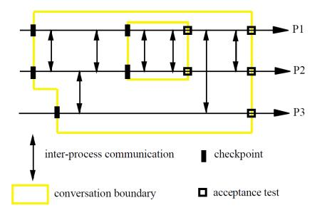
The operation of a conversation is: (i) on entry to a conversation a process establishes a checkpoint; (ii) if an error is detected by any process then all the participating processes must restore their checkpoints; (iii) after restoration all processes use their next alternates; and (iv) all processes leave the conversation together.
