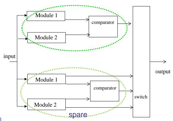
Pair results are used in a spare arrangment. Spare components at coarser granularity Not all four copies must be synchronised (only the two pairs)
