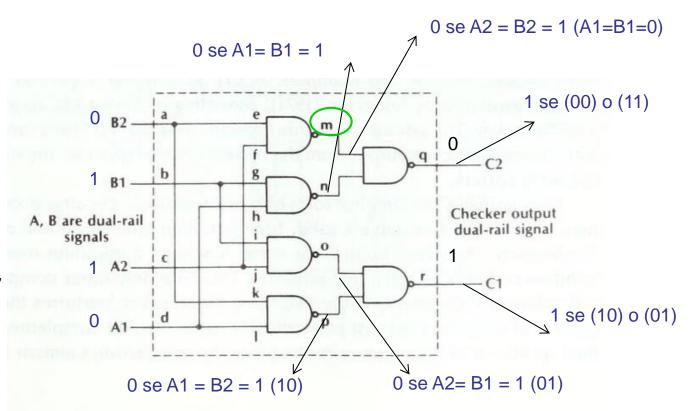
Set of faults: stuck-at-1, stuck-at-0 of each line (a, b, c, d, e, ....., q, r) Fault free A =0, B =1 m=1, n =1, q=0 o = 0, p=1, r= 1 c2=0 c1=1 code different input
