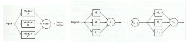
A complex system can be partitioned into smaller subsystems The effect of partitioning of modules (A, B, C) is that the design can withstand more failures than the solution with only one large triplicated module
