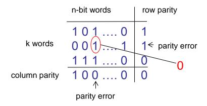
Error location is possible for single-bit error: one error in the row parity vector, one error in the column parity vector
