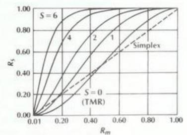
Figure 2. system with standby failure rate equal to 10% of on line failure rate
