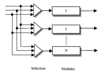
Figure 15: Passive Redundancy with Input Voting
