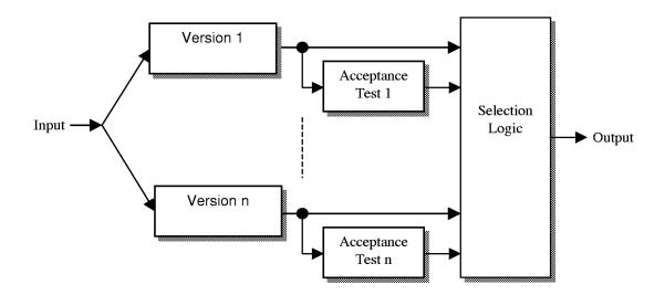
Figure 11: N Self-Checking Programming using Acceptance Tests
