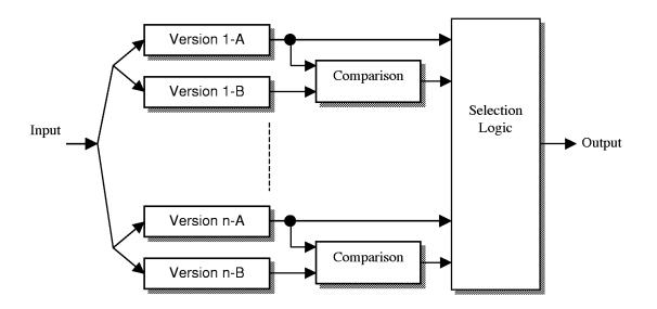
Figure 12: N Self-Checking Programming using Comparison
