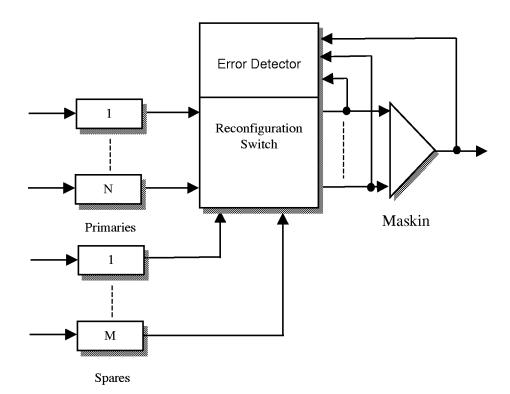
Figure 18: Hybrid Redundancy using N-Modular Redundancy with Spares
