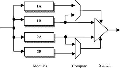
Figure 17: Dynamic Redundancy using Self-Checking Pairs
