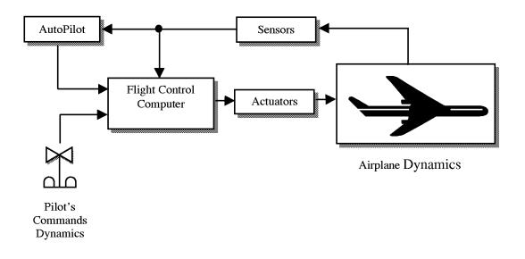
Figure 19: Abstract Representation of a Fly-By-Wire Flight System
