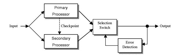
Figure 4: Logical Representation of Process Pairs
