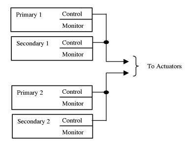
Figure 21: Architecture of A3XX Flight Control Computer
