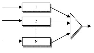
Modules Selection Figure 14: Example of Passive Redundancy
