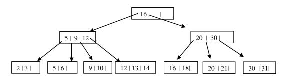
Show the form of the B+-tree after each operation of the sequence: Delete 18; Delete 31; Insert 15.
