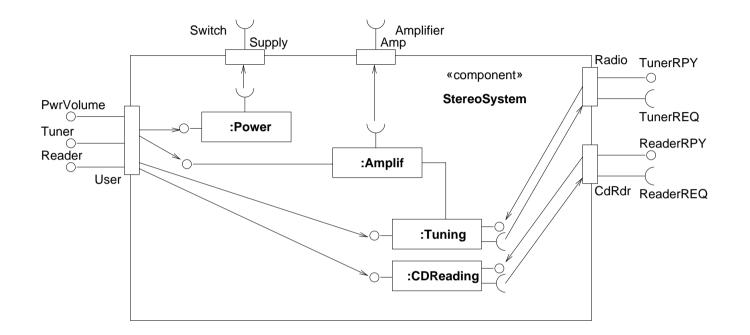
Internal structure of the component.
