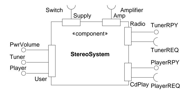
Switch, Amplifier, TunerREQ, PlayerREQ: *required* interfaces (sets of operations called by the component) PwrVolume, Tuner, Player, TunerRPY, PlayerRPY: *provided* interfaces (sets of operations called by other components)
