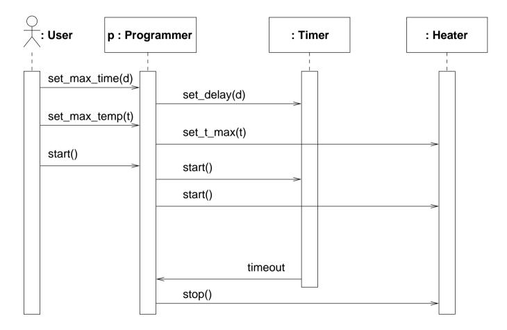
Scenario 2: timeout occurs before the heater reaches the limit temperature.
