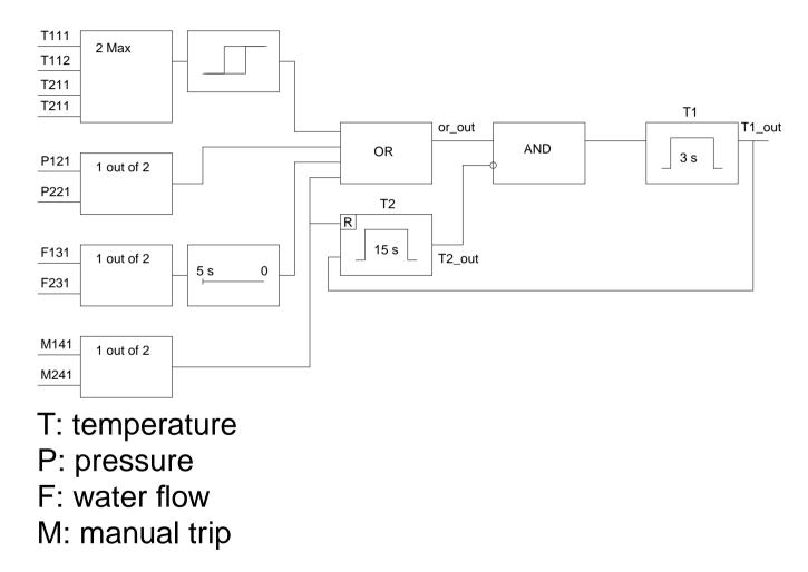
(adapted from K. Björkman et al., Verification of Safety Logic Design by Model Checking, NPIC&HMIT 2009)
