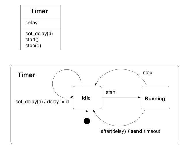
after(...): fire transition after *delay* seconds (*time event*) send: generate a timeout *signal*
