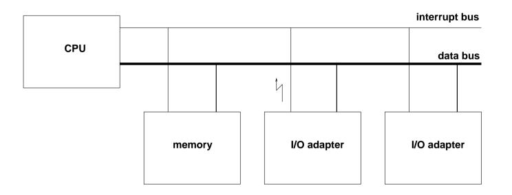
*External interrupts* are signals that peripheral devices send asynchronously to the CPU on the occurrence of some events, such as completion of a HW operation, availability of input data, HW faults...
