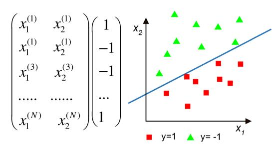
Target: find the correct weight set  $(w_1, w_2)$  and bias *b* that allow the perceptron to predict the label on a new data. In the case shown above, the data are "linearly separable", i.e. a line exists that divide the  $x_1, x_2$  plane into two regions where points with homogeneous label are present
