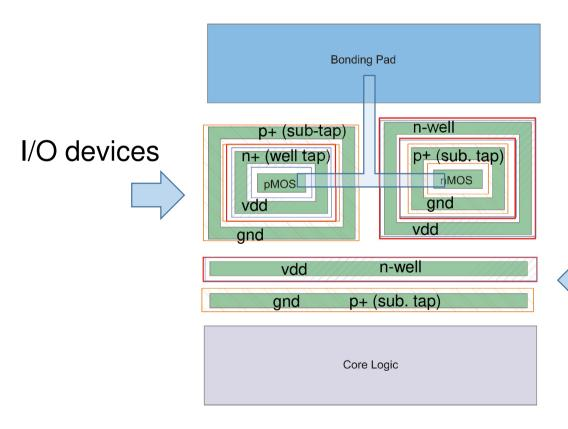
Guard rings are placed around the I/O devices in order to:
