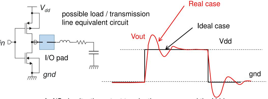
In I/O circuits, the output termination can exceed the Vdd or gnd rails. This introduces additional risk of latch-up
