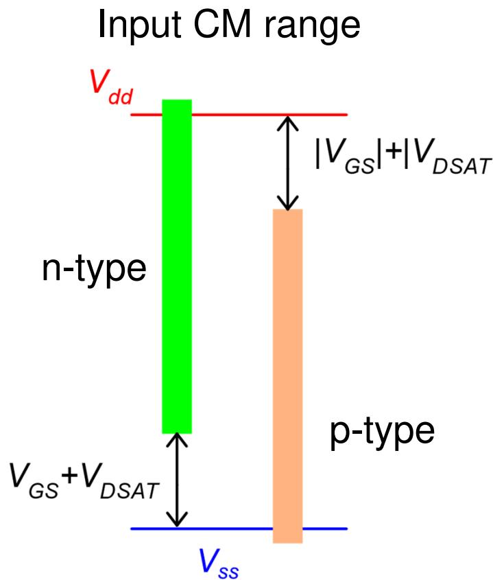
The idea is to make an n-type and p-type OTAs work together,
