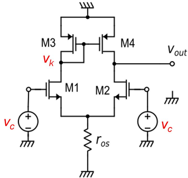
It is possible to exactly calculate  $i_{occ}$ , taking into account the actual  $i_{d1}/i_{d2}$  ratio and  $i_{d4}/i_{d3}$  ratio ....
