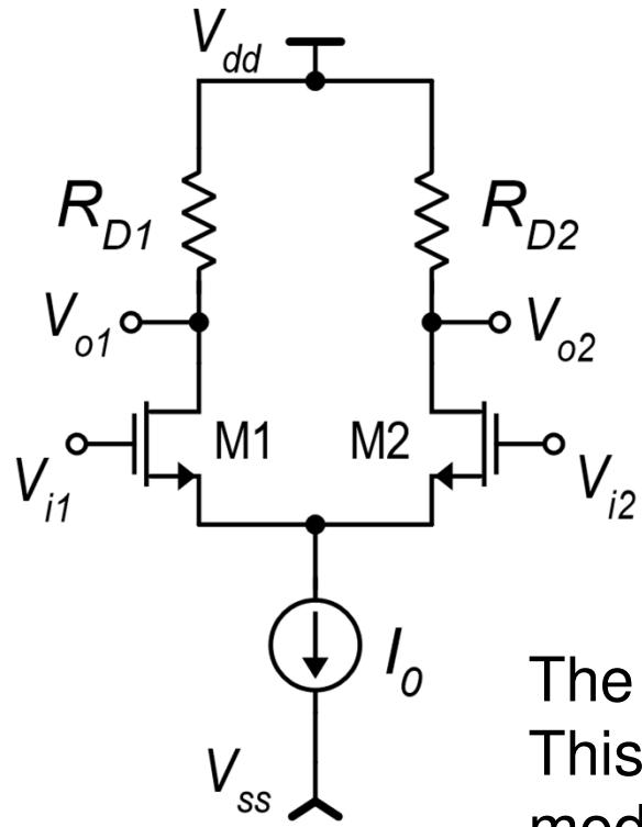
1. The S/E version has a poor CMRR (large  $A_c$ ) and large input offset voltage
