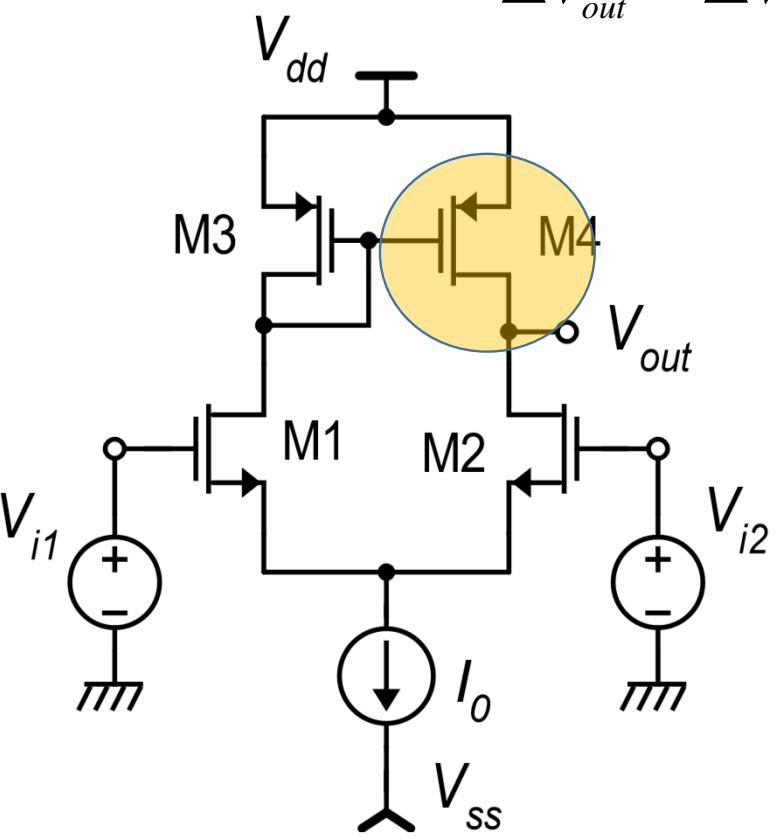
$$\Delta V_{out} = \Delta V_D R_{out} (V_{DQ}) \left( \frac{dI_{occ}}{dV_D} \right)_{V_D=V_{DQ}}$$
