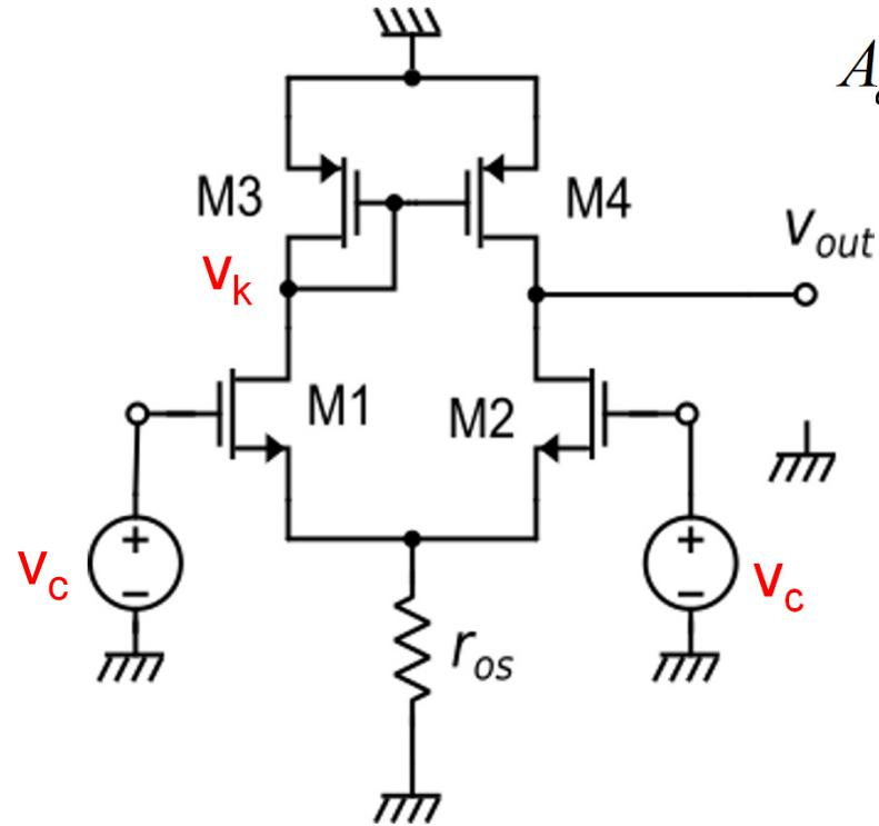
$$A_c = \frac{v_{out}}{v_c} \Big|_{v_d=0} = -\frac{1}{2g_{m3}r_{os}} \quad A_d = \frac{v_{out}}{v_d} \Big|_{v_c=0} = g_{m1}(r_{d2} // r_{d4})$$
