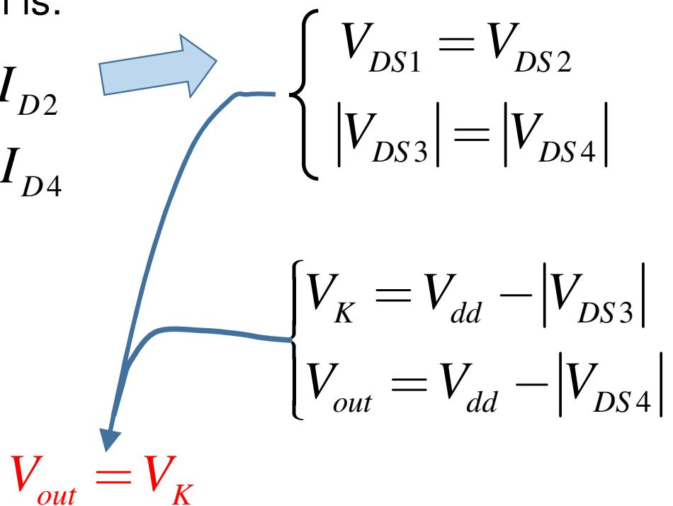
For  $V_{id}=0$ , the electrical solution is perfectly symmetrical
