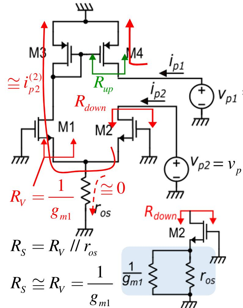
Case 1:  $v_{p1} = v_p, v_{p2} = 0 \rightarrow i_{p1} = i_{p1}^{(1)}, i_{p2} = i_{p2}^{(1)}$
