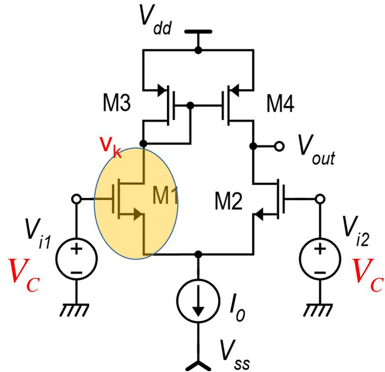
As  $V_C$  is progressively increased, also  $V_S$  increases at the same pace. Since  $V_{out} = V_K = V_{D2} = V_{D1}$  is fixed, eventually  $V_{DS1}$  and  $V_{DS2}$  will drop below the saturation voltage.
