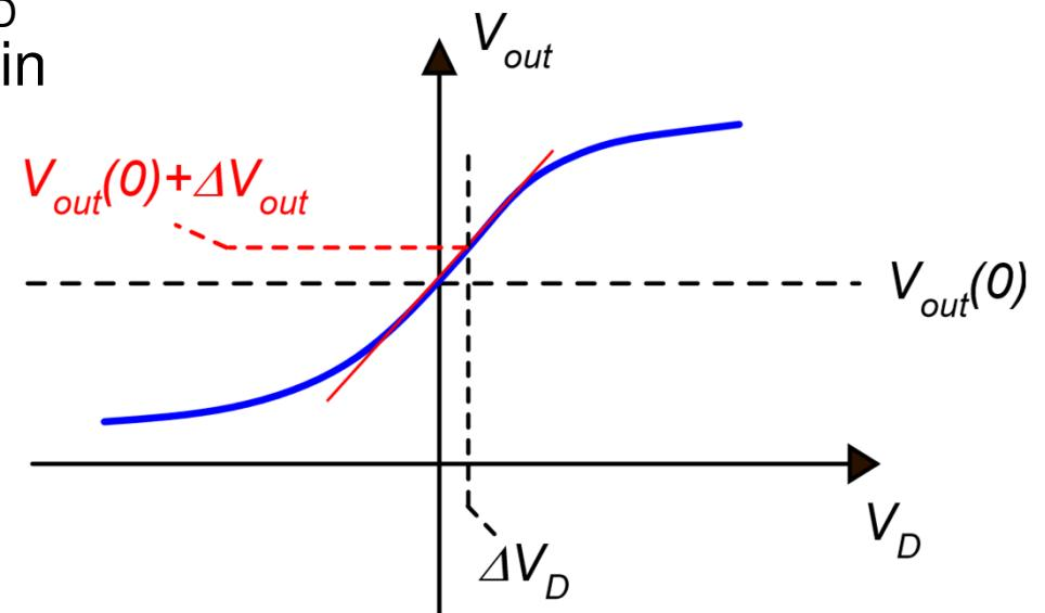
$$\Delta V_{out} = R_{out} \Delta I_{OCC}$$
