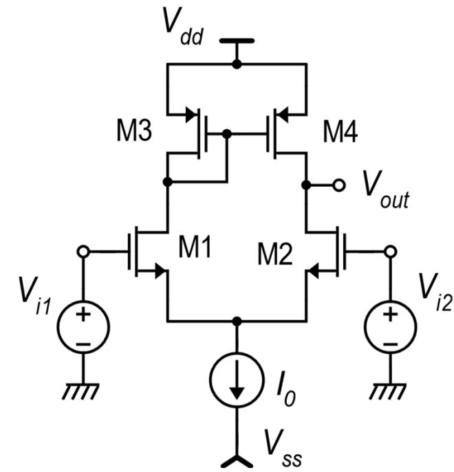
$$V_{dd} - |V_{GS3}| + V_{GS1} - V_{DSAT1} \geq V_C$$
