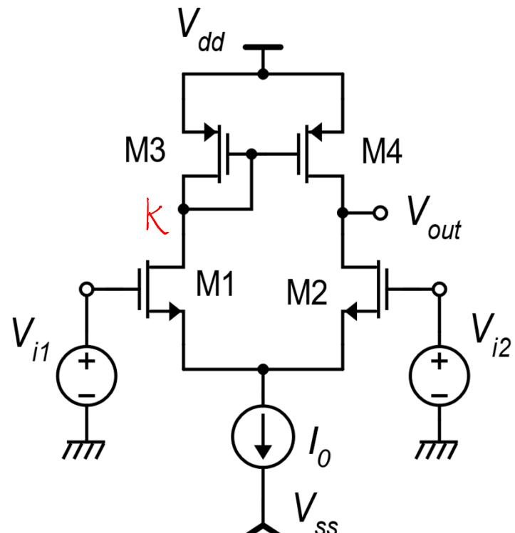
$$V_{i1} = V_C + \frac{V_D}{2} \quad V_{i2} = V_C - \frac{V_D}{2} \quad V_C = \text{constant}$$
