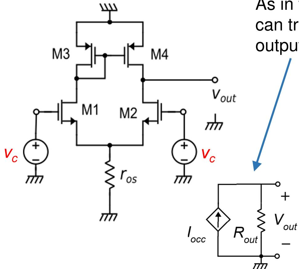
$$v_{out} = i_{occ} R_{out} \quad R_{out} = r_{d2} // r_{d4}$$
