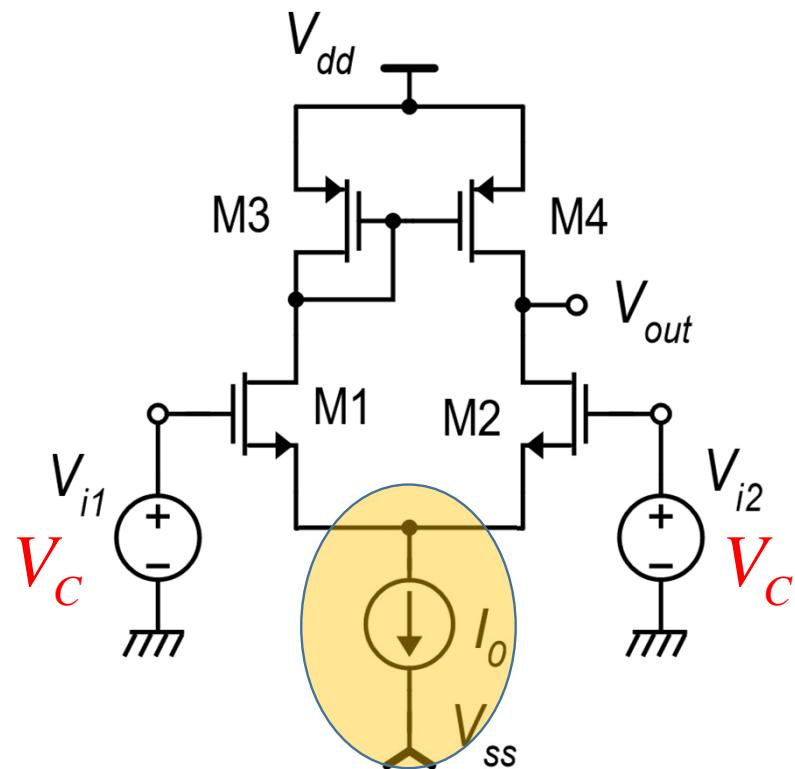
As  $V_C$  is progressively decreased, also  $V_S$  decreases at the same pace and eventually the voltage across the current source  $I_0$  will get smaller than the minimum value  $V_{MIN}$ . From that point on,  $I_0$  will rapidly decrease, turning off the stage.
