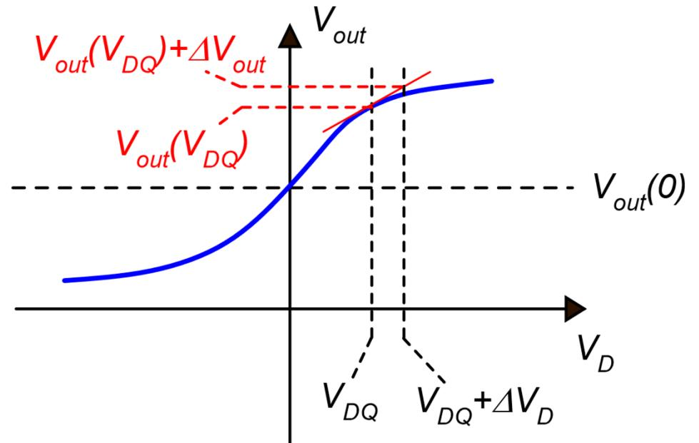
$$\Delta V_{out} = \Delta V_D R_{out} \left( V_{DQ} \right) \left( \frac{dI_{occ}}{dV_D} \right)_{V_D=V_{DQ}}$$
