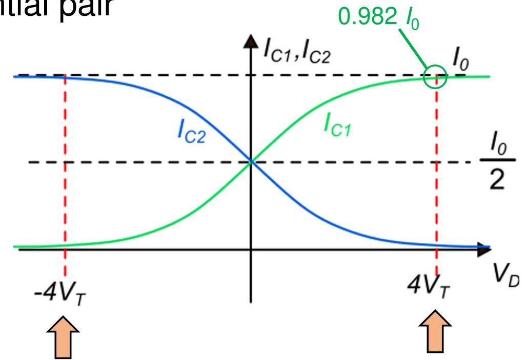
$$I_{C1} - I_{C2} = I_0 \frac{1 - e^{\frac{-V_D}{V_T}}}{1 + e^{\frac{-V_D}{V_T}}}$$
