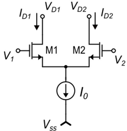
$$x = \frac{1}{2} \pm \frac{1}{2} \sqrt{2 \left( \frac{V_D}{V_{DMAX}} \right)^2 - \left( \frac{V_D}{V_{DMAX}} \right)^4} = \frac{1}{2} \pm \frac{1}{2} \left( \frac{V_D}{V_{DMAX}} \right) \sqrt{2 - \left( \frac{V_D}{V_{DMAX}} \right)^2}$$
