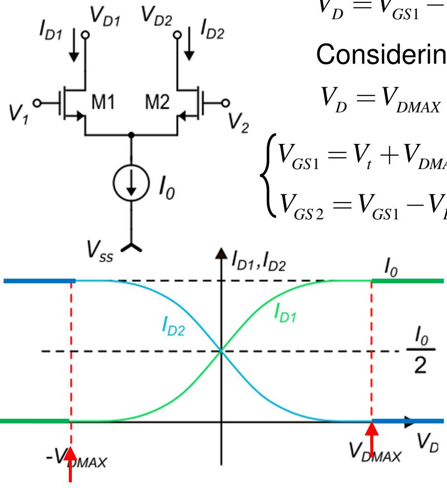
$$V_D = V_{GS1} - V_{GS2} \Rightarrow V_{GS2} = V_{GS1} - V_D$$
