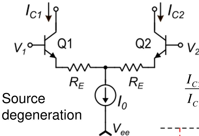
$$g_{m-rid} = \left. \frac{d(I_{C1} - I_{C2})}{dV_D} \right|_{V_D=0}$$
