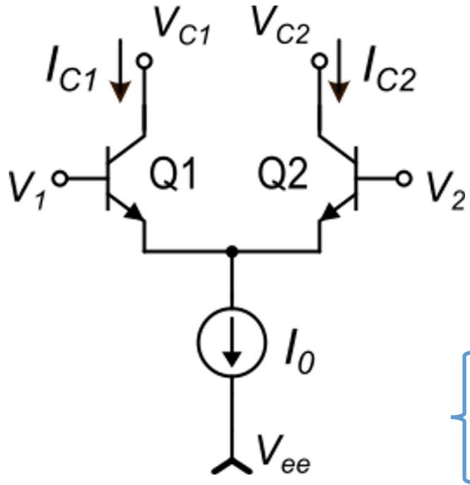
$$I_{E1} + I_{E2} = I_0 \quad \Rightarrow \quad \frac{\beta+1}{\beta} I_{C1} + \frac{\beta+1}{\beta} I_{C2} = I_0$$
