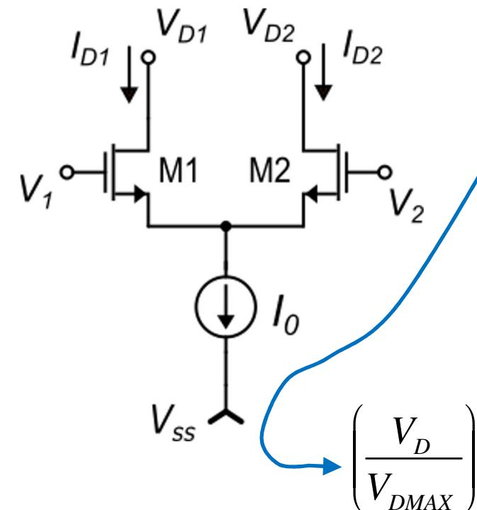
$$\frac{V_D}{V_{D\text{MAX}}} = \left[ \sqrt{x} - \sqrt{(1-x)} \right]$$
