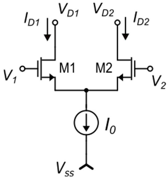
$$I_{D1} - I_{D2} = I_0 \left( \frac{V_D}{V_{DMAX}} \right) \sqrt{2 - \left( \frac{V_D}{V_{DMAX}} \right)^2}$$
