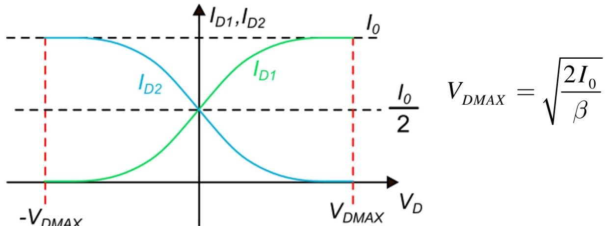
For  $V_D=0$  (typical operating point):  $I_{D1} = I_{D2} \triangleq I_{DQ} = \frac{I_0}{2}$
